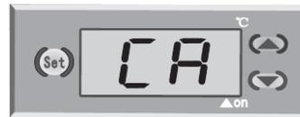
Hold "set", then press ▲ or ▼ simultaneously. Choose temperature correction: -15°C to 15°C
